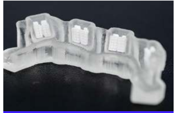
Closeup of LightForce's 3D printed custom dental braces and tray.
